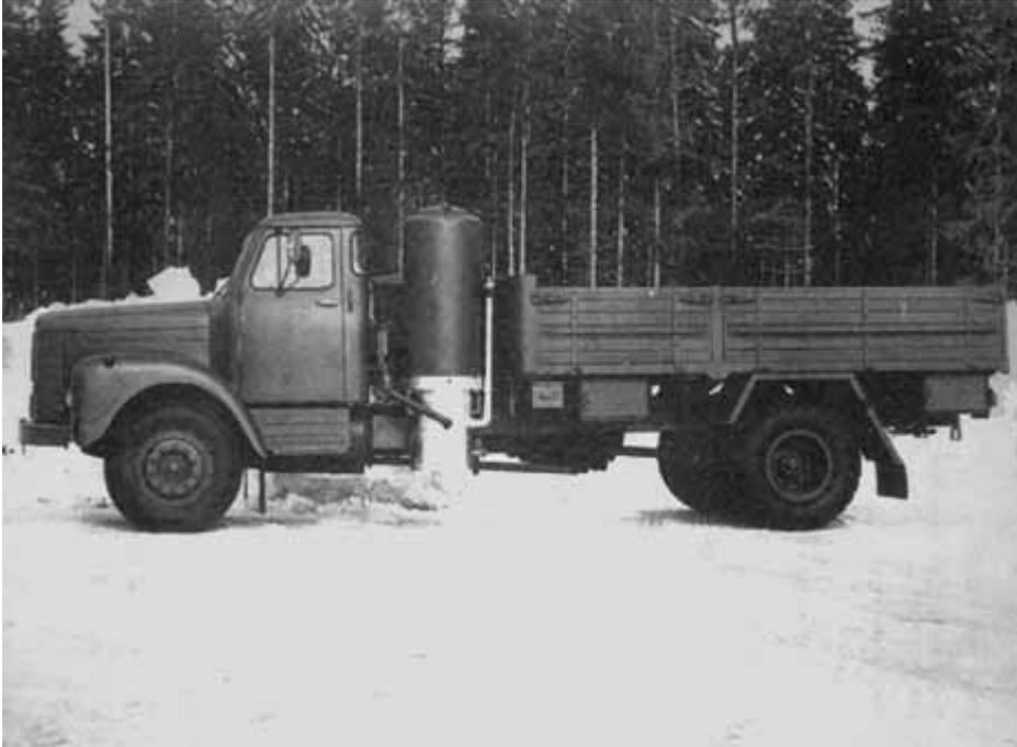
Table 3.14 Specification of Scania truck converted to producer gas
