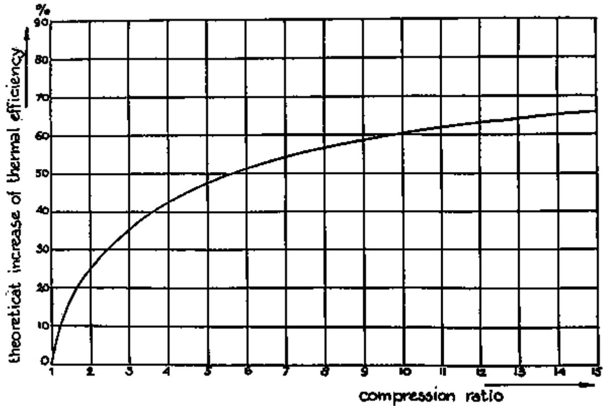
Figure 2.2 shows the influence of compression ratio on maximum engine power output.
