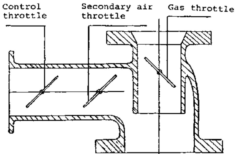
**Figure 3.14 Gas air mixers tested for the Scania L8050 truck - b. Gas-air mixer designed by the National Testing Institute for Agricultural Machinery**
