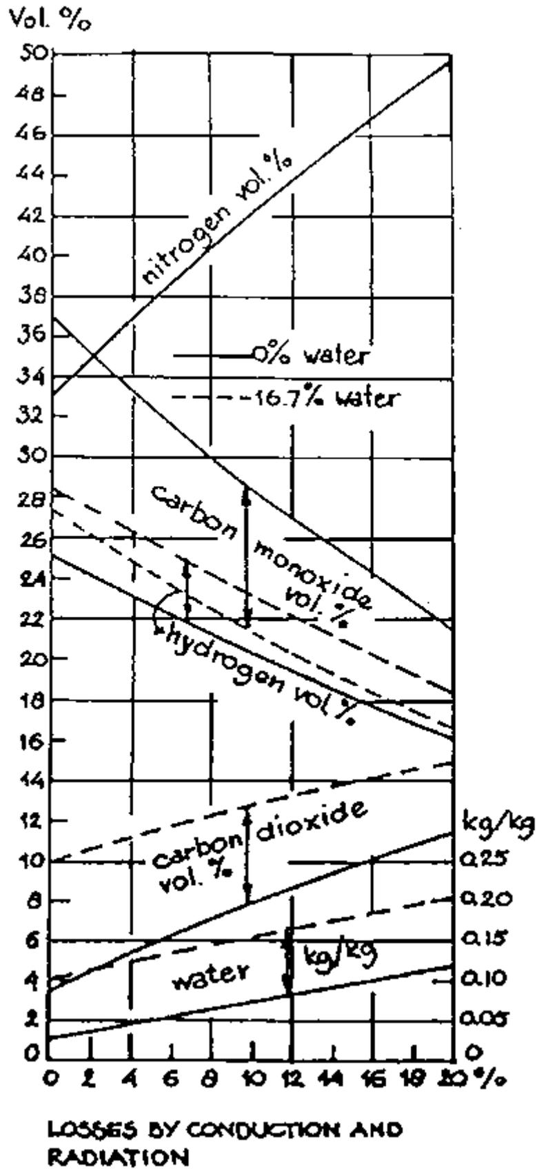
Figure 2.6 Calculated change of woodgas composition as a function of the gas outlet temperature (losses through sensible heat)
