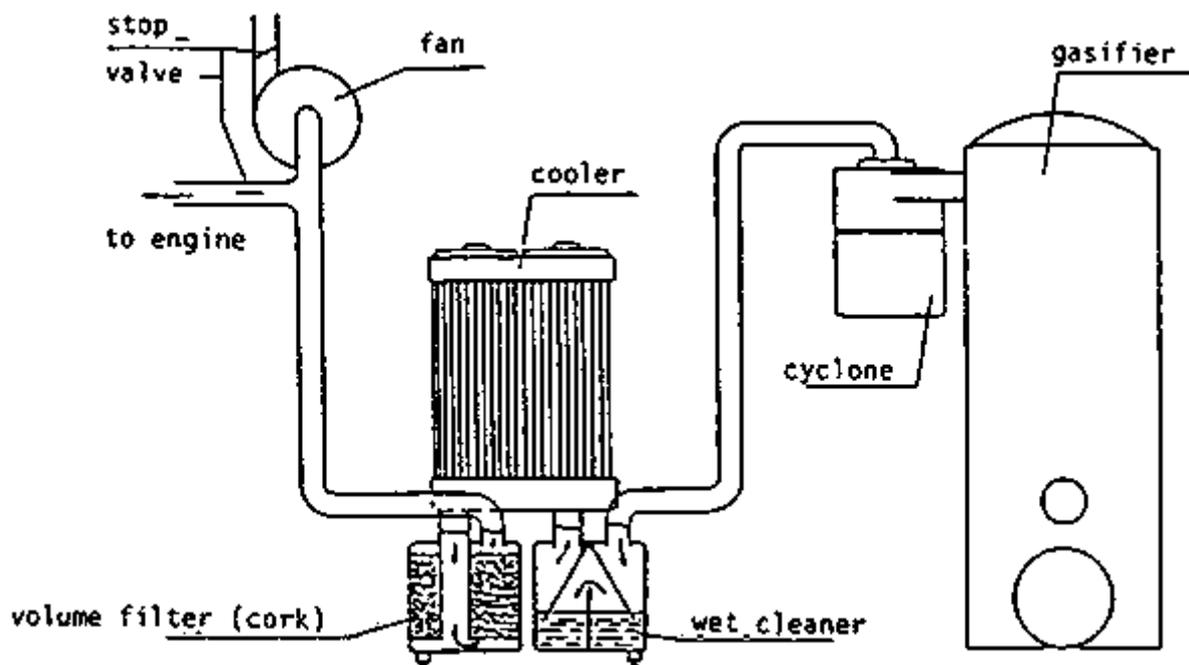
**[Figure 3.5 Gas cleaning systems for vehicles tested by Nordstrom \(33\) - b. Fabric filter cleaning system with cyclone.](#)**
